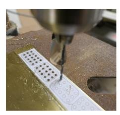
Drill the holes with a 2mm drill bit
