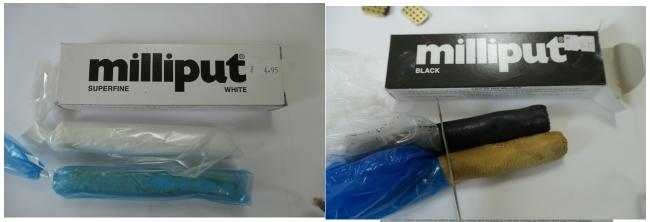
Cut an equal length off each part and mix the two parts together
