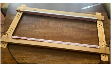
The width of the work that can used in the frame is determined by the space between the slots on the support bar. Ideally, I would ideally have a minimum 4-6in gap between the edge to work and the spacer bars. This determines the length of support bars.
